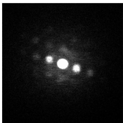
Figure 7. Convergent beam electron diffraction pattern (CBED) of 20–30 nm PtBi nanocrystalline networks
